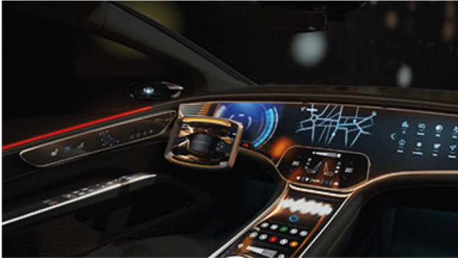
Figure 2: Dynamic light for warning a driver or passenger
